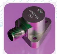
Industrial grade vibration transducers. Signal output is floating, via 2 pole hermetic connector, thus minimizing common mode interference. Ingress of contaminants into the transducer and/or connector will degrade data. Transducers and cables can be supplied proof pressure tested to 80bar, individually and as assemblies.
